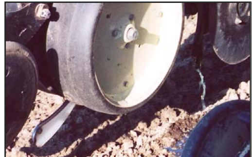
Placement 1 inch to the side of the seed furrow with fertilizer disk.
