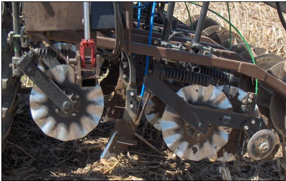
Nutri-Till applicator in the raised position showing placement of the nitrogen (blue tube) and Pro-Germinator , Sure-K and micronutrients (green tube).
