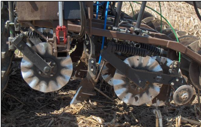
Nutri-Till TM in the raised position showing dual placement of liquid fertilizers.
