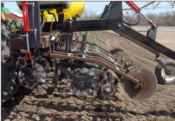
Nutri-Till™ implement in the raised position.
