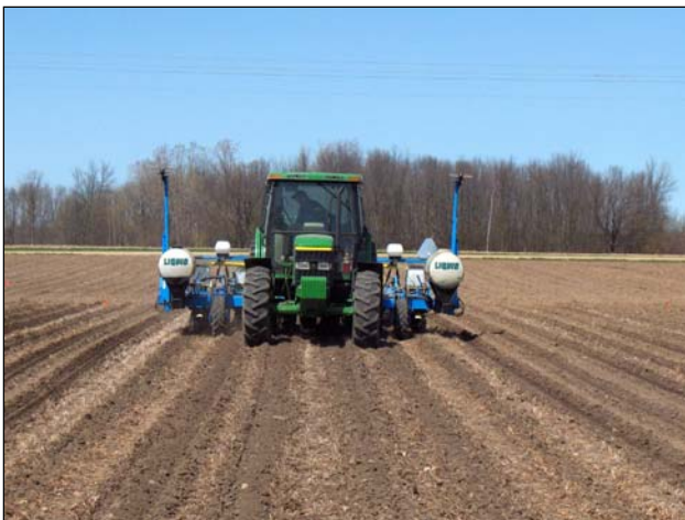
Planting over the Nutri-Till™ strips leaving wheat stubble residue between the rows.
