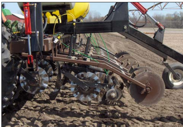
Nutri-Till™ implement in the raised position.
