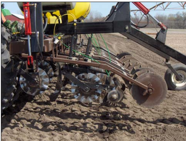
Nutri-Till TM implement in the raised position.
