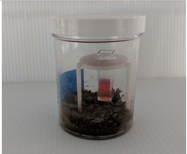
Figure 2. A Cuvette with gel in a standard measurement of the CO 2 released by basal soil microbial respiration in Lab. conditions. Gel absorbance (Abs. T 0 - Abs.T 24 ) is measured after calibration with blank cuvette.
