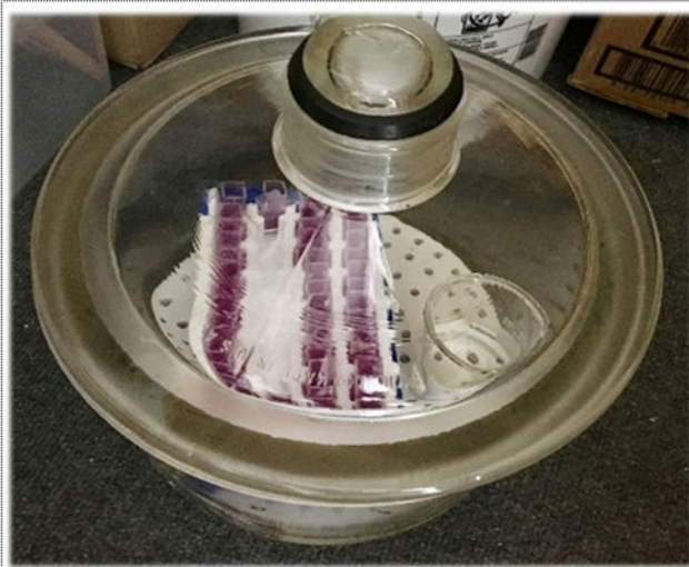
Figure 1. Cuvettes are kept in a desiccator in the dark at room temperature with an excess of soda lime and water for one week to absorb atmospheric CO 2 .
