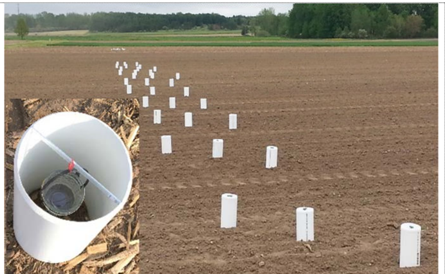
Figure 1. Passive sampler for CO 2 capture spread across a research field at AgroLiquid (2017).
