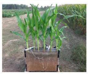
Soil monolith representing suction of soil liquids by Micro-Lysimeters for measurements of active phosphorus in soil.
